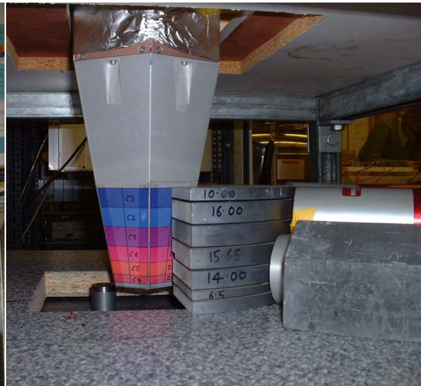
Liverpool coincidence setup with multileaf collimator partial scan of first prototype (spring 2005)
