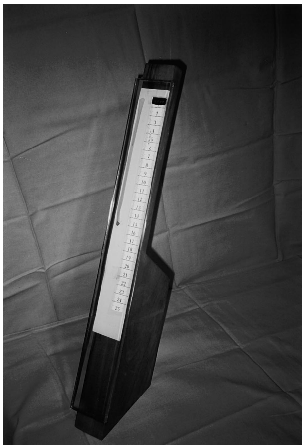
Fig. 1. Home-made anticoagulation monitor (HACOM) after tilting the wooden frame by 65.5°. In this position, the blood drop was running down longer or shorter, depending on the degree of anticoagulation.
