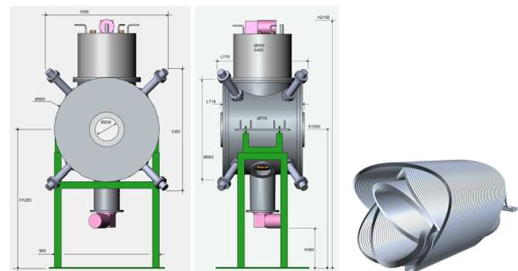
Figure 1: View of MAGDEM fully-integrated system and only magnetic coils.
