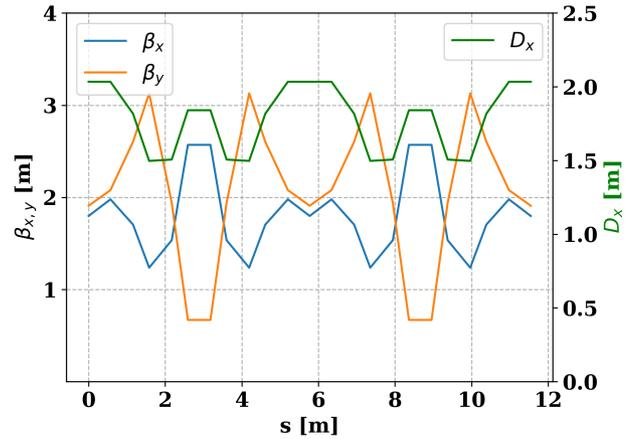
Figure 3: Betatron functions ( $\beta_{x,y}$ ) and first order horizontal dispersion function ( $D_x$ ) in the ISRS ring operating in isochronous mode.
