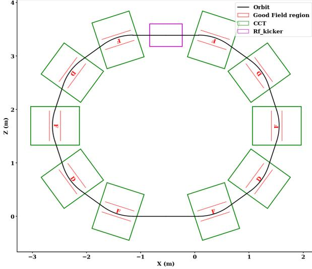
Figure 2: Floor layout of the ISRS ring.
