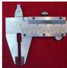
PIE DE REY DONDE SE APRECIAN LAS PARTES PARA MEDIR DIMENS. INTERNAS Y EL NONIO.
