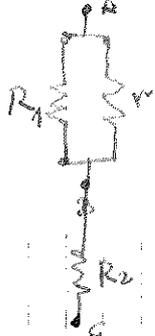
$$V_A - V_B = \frac{R_1 r}{R_1 + r} \cdot \frac{E}{R_2 + \frac{R_1 r}{R_1 + r}} = \frac{E}{1 + \frac{(R_1 + r)R_2}{R_1 r}} = \frac{E}{\frac{R_2 + \frac{R_2}{r} + 1}{R_1}} = \frac{E R_1}{R_2 + \frac{R_2}{r} + 1}$$
